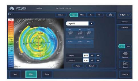
Through data collection and analysis, VX105 can generate different kinds of maps to support evaluation of cornea health such as bi-focal axial map, tangential map, refractive map, elevation map, difference map and etc.
